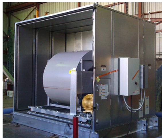
Daikin Vision® air handler OSHPD pre-approval seismic testing on the University of California, Berkeley Pacific Earthquake Engineering Research (PEER) shake table.
