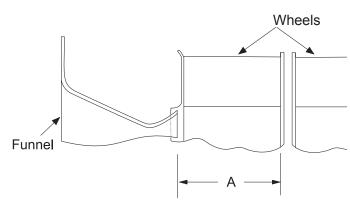
Figure 78: 40" SWSI Airfoil Wheel-to-Funnel Alignment
