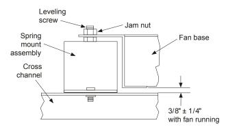
\* Grossly out-of-adjustment thrust restraints can affect this dimension. Recheck after thrust restraints are adjusted.
