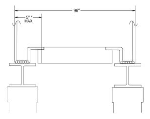
\* Beam can extend beneath unit no more than 5" to allow adequate space for duct connections and electrical entry.
