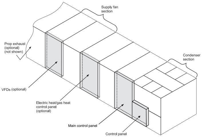
Figure 11: Typical Main Control Panel, 460 Volt
