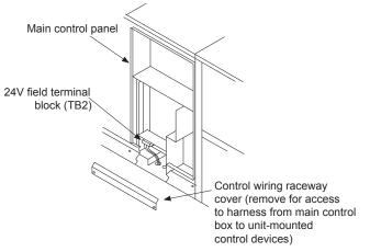
Figure 36: Control Wiring Raceway
