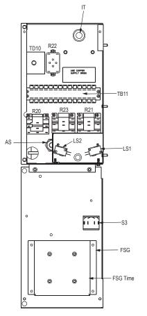
Figure 14: Condensing Unit Control Panel
