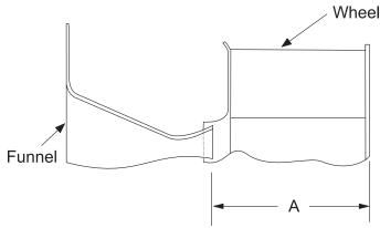
Figure 77: DWDI Airfoil Wheel-to-Funnel Alignment
