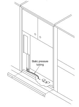
Figure 31: Pressure Sensing Tubing Installation
