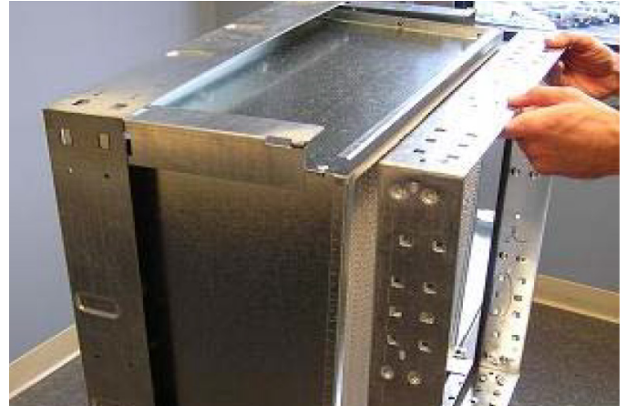
Figure 42: Positioning of the prefilter frame
