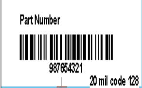
NOTE: This label should also include a lot identifier as noted in specification (for traceability in case of quality recalls etc.... Could be date code, serial number, lot ID, etc....
