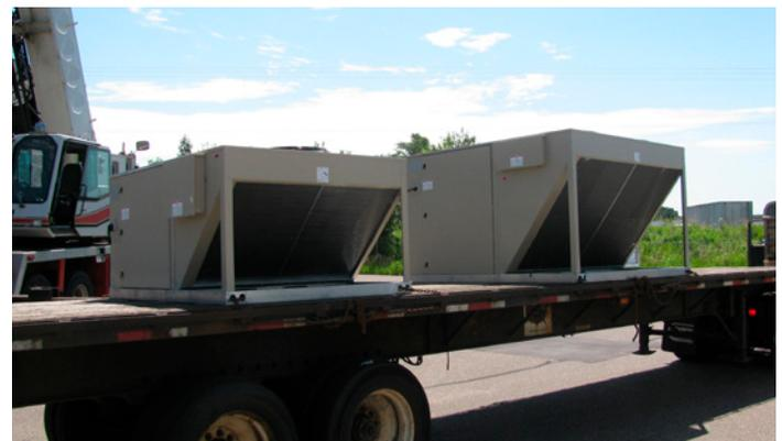
*Two 10-ton Rebel rooftop systems with variable speed compressors and EC fan motors were specified for Phase 2 of the Regatta project.*
