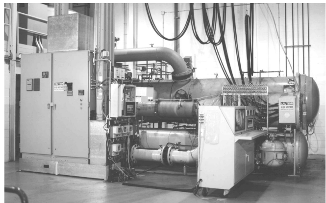
Figure 7: McQuay's million-dollar compressor test stand with advanced data acquisition provides comprehensive information on new compressor designs.
