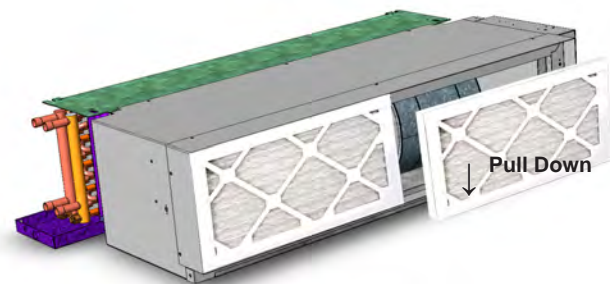
Figure 17: Filter Removal for Units with Rear Returns
