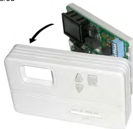
Figure 2. Pull left end of cover away until tabs at right end are cleared
