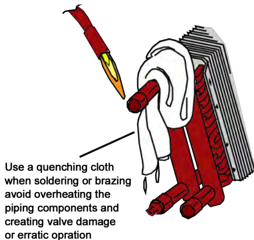
Figure 6: Protect Components from Overheating
